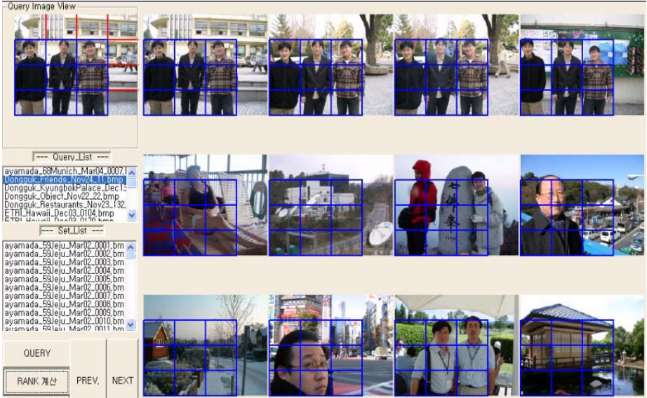
Fig. 4. Imageretrieval with the combined EHD and CLD (query image: upperleft-most, ROI: lower left 3 \times 3 sub-images, ranking: raster scan order).
